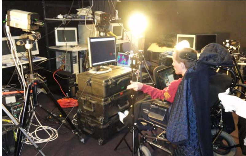
Fig. 6. Experimental setup. The user is placed in front of a computer screen with a webcam capturing his motions to enable mouse pointer control. We simultaneously recorded his motions with a two-camera thermal infrared system and a high-speed four-camera visible-light system for future analysis.
