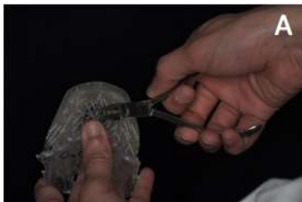
A) After post curing the support area was removed with pliers. B) The excess PUT was removed in the same way.
