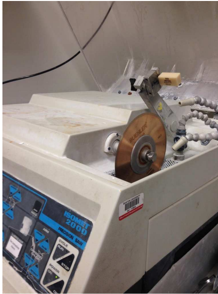
Figure 3: Precision saw used to cut CAD/CAM blocks into identical sized tiles.
