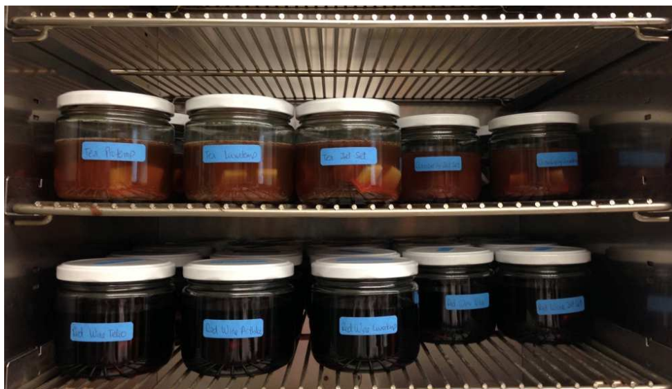
Figure 5: Specimens immersed in different beverages in sealed jars at the incubator at 37 °C.
