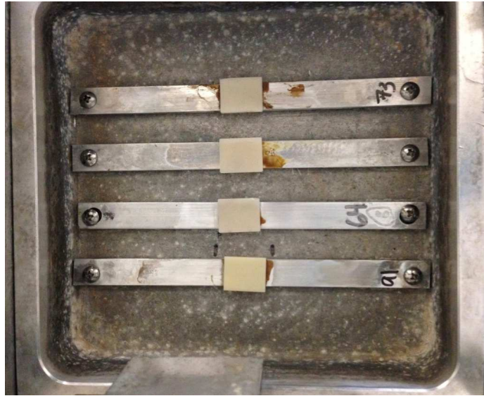
Figure 8: Lower compartment of simulated tooth brushing machine, holding the specimens in bars attached with sticky wax.
