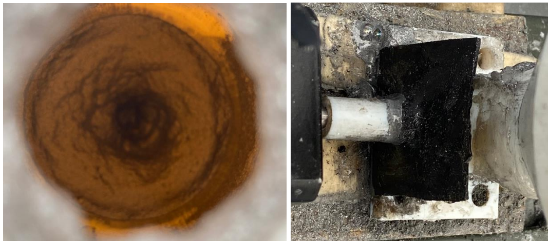
Figure 35: Aluminum Left in Reactor (left) and Leaking of the Pump (right)
