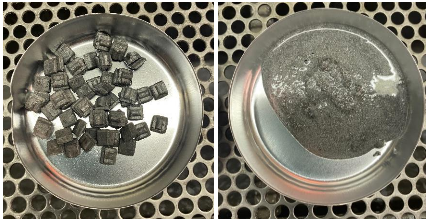
Figure 5: Activated Aluminum Chips (left) and Slurry (right)
