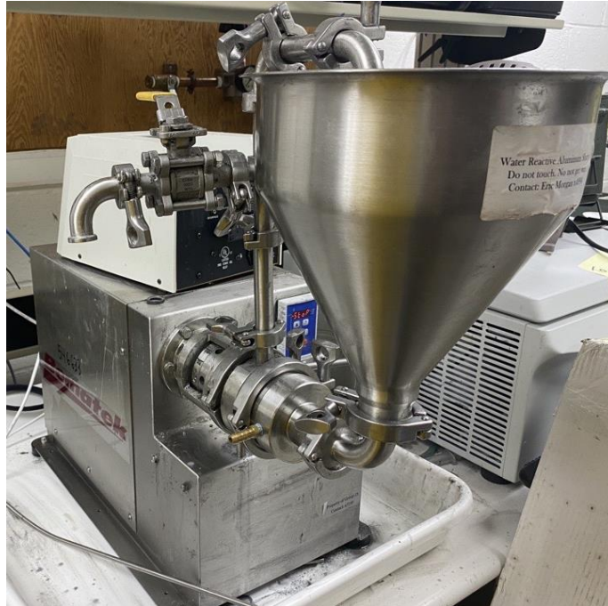
Figure 9: Colloid Mill Used for Producing Aluminum Slurry
